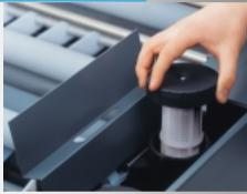
The placing of the developer filter right under the top cover allows it to be removed easily. It also means that the tank system does not need to be emptied prior to filter removal. An optional range of filters meets all applications and needs.
