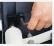
The snap lock system makes removal of the rollers a very easy operation.
