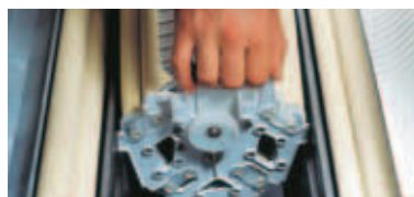
Easy maintenance Rack mounted modules make it easy to disassemble the processor for maintenance.
